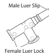
\*Tee with female luer lock on two sides and male luer slip on one side
